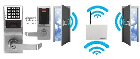
Up to 2000 locks \*\*and a computer communicate wirelessly through bidirectional Gateways - eliminating the need for door-to-door programming and audit trail retrieval.
